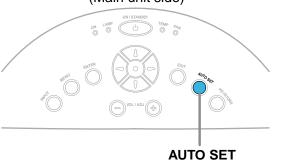
You can adjust the optimum horizontal position, vertical position, sampling phase and sampling frequency for projecting analog RGB signals at the touch of a button.
